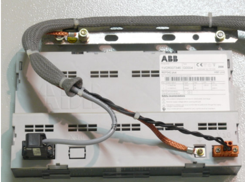
Figure 6.4.4: Earthing connection for separated HMI
